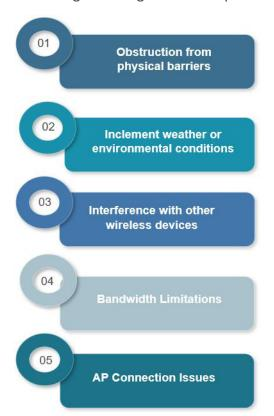
**SOLUTION:** Mount wireless antennas above obstruction or transmit around the obstruction. When transmitting around the obstruction, install repeaters along with new wireless transmitters around obstacles so that points to points can bounce from one repeater to another to get to a gateway or its destination.
